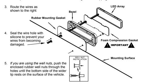
6. Review the mounting diagram and use the appropriate screws to mount the bezel.
